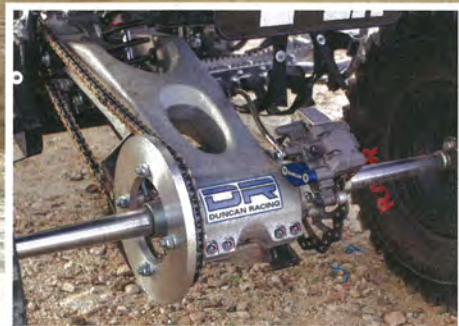
A stock swingarm utilizes a Roll Design linkage to attach the Elka shock to the YFZ. An RPM Dominator II axle replaced the stock one. DR protection, Sunstar sprockets and a RK Excel chain were installed.
