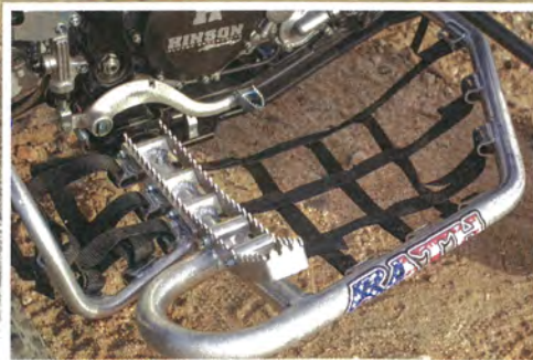
Rath Racing competition nerf bars with their monster peg found a home on this machine. There is plenty foot traction available. Some Hinson components were installed as well.
