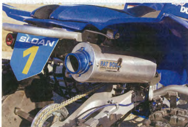
A large increase of exhaust flow is due to Duncan's Fat Boy 4 stainless steel full exhaust system.
