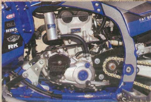
Duncan Racing's oil catch can keeps the Yamaha engine from blowing out too much oil during rough riding. The Zip high-capacity oil cover offers 8.5 more ounces of capacity, and the Works Connection engine plugs are a nice touch.
