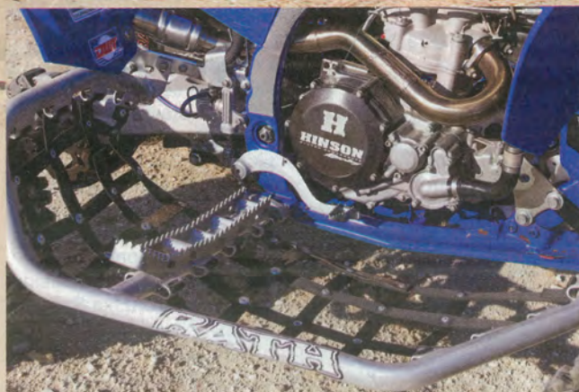
Rath Racing's Signature Series nerf bars are very protective, and their Monster peg has sharp teeth for great foot traction. Hinson's clutch kit is an impressive addition.
