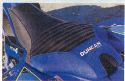
Zip's Pro Top seat cover has grippy material on the sides and ridges on top that help keep the rider in place. Yamaha's slim body makes moving around the quad easy.
