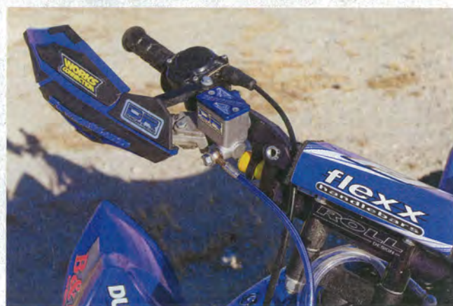
Fastt Co. Flexx bar smooths out vibrations with ease. The Works Connection brake reservoir cap is a nice touch, and the Powermadd guards protect Mike's hands.
