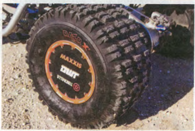
Sloan prefers to run a Maxxis RAZR XC tire. The DWT beadlock wheels are used by many racers due to their strength and ease of maintenance.
