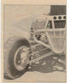
Long enough A-arms for you? The final width is 2" wider than stock. Though this machine uses stock Honda brakes, the Pro-Trax T-pin spindles can also be designed for Banshee brakes.
