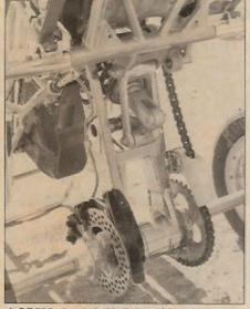
A CR500 shock (with linkage) has become the hot setup on FourTraxes and it makes sense to run it on the Banshee, too. Notice Laeger's brake rotor guard and the Hondastyle axle carrier and chain adjustment.
