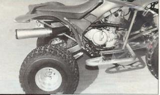
Duncan Racing outfitted both machines with Holeshot tires, AC aluminum grab bars and nerfs, as well as Cascade seat covers. Nice! Though Duncan is developing its own exhaust systems, it favors SuperTrapp among those currently available. For stability, both the Warrior and EX received RPM Dominator axles.
