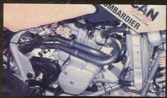
You can be sure the final production Duncan headpipes will have nice welds and will be stainless steel. Of course, the performance gain, which is substantial in the bottom end, will still be there.
