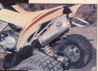
Duncan's muffler for the DS produced a deeper tone than the stocker. A tuncable bolt-on spark arrestor is available from Duncan Racing.
