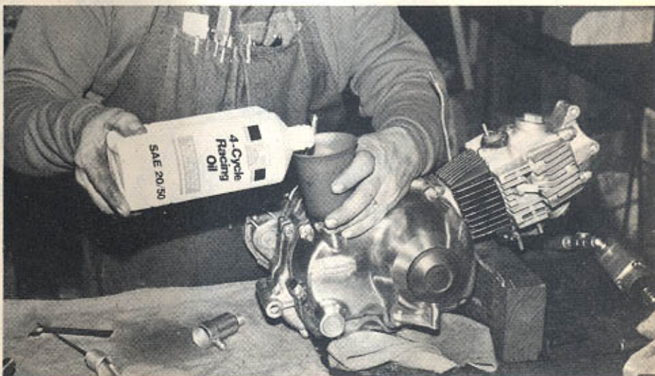
ABOVE, during all tests run on the ATC 90 engine, Bel-Ray 20/50, 4-cycle Racing Oil was used. The ATC engine takes one quart of oil to reach the full mark. Nice looking polished side covers came from Johnson's ATC in Santee, Calif.
