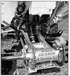
The rear end is modified to use a Braking rear disc from Honda TRX250R with an ATV Innovations rear caliper. This mod improves ground clearance and improves braking performance.
