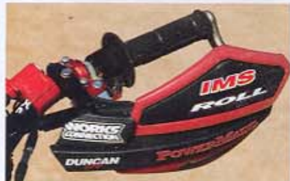
A Works Connection clutch perch, PowerMadd handguards, the required tether killswitch, a toggle for the Vortex two-curve ignition and a twist throttle belly up to the bars.
