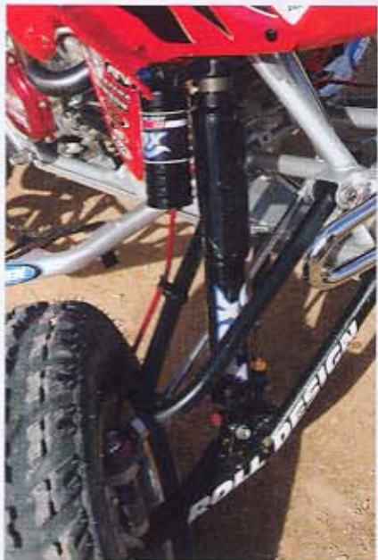
Roll Designs A-arms widen the DRI 450R by four inches, and the Fox Float XI airshocks provide practically infinite tuning adjustments.
