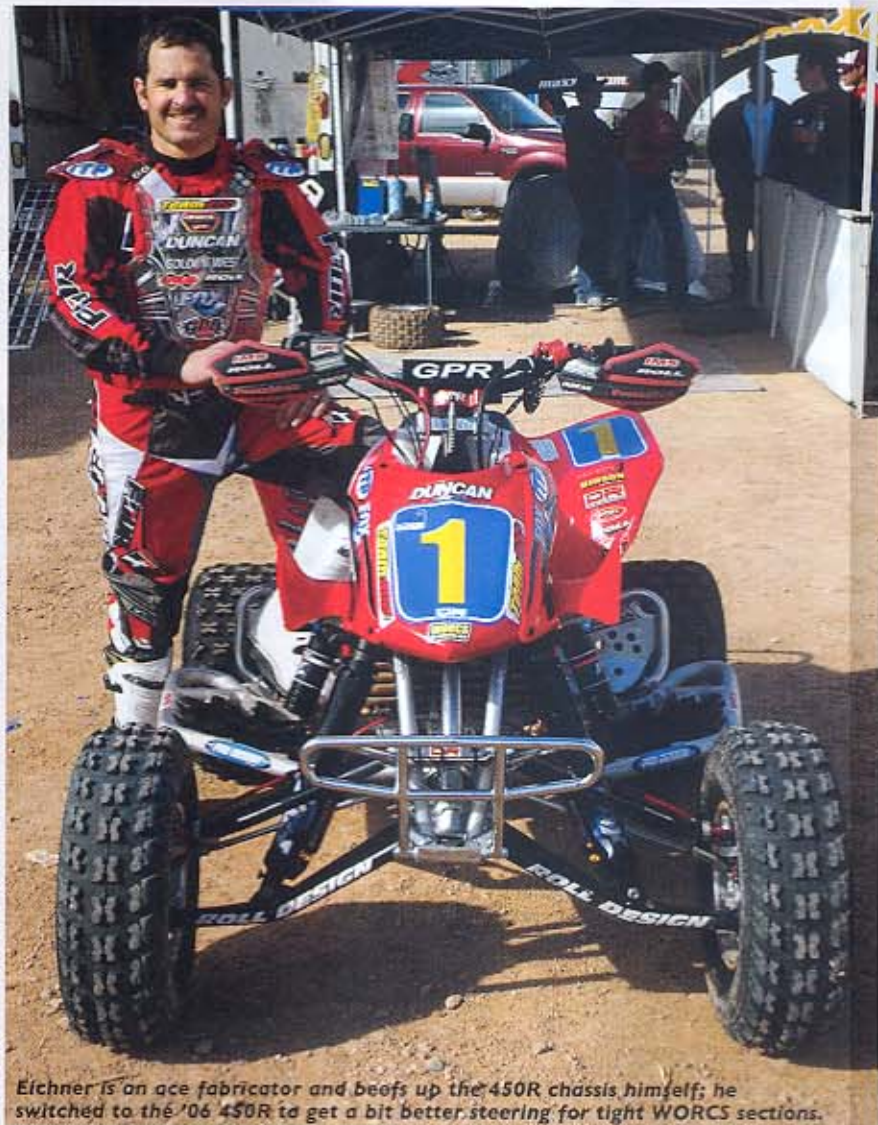
A Works Connection clutch perch, PowerMadd handguards, the required tether killswitch, a toggle for the Vortex two-curve ignition and a twist throttle belly up to the bars.
