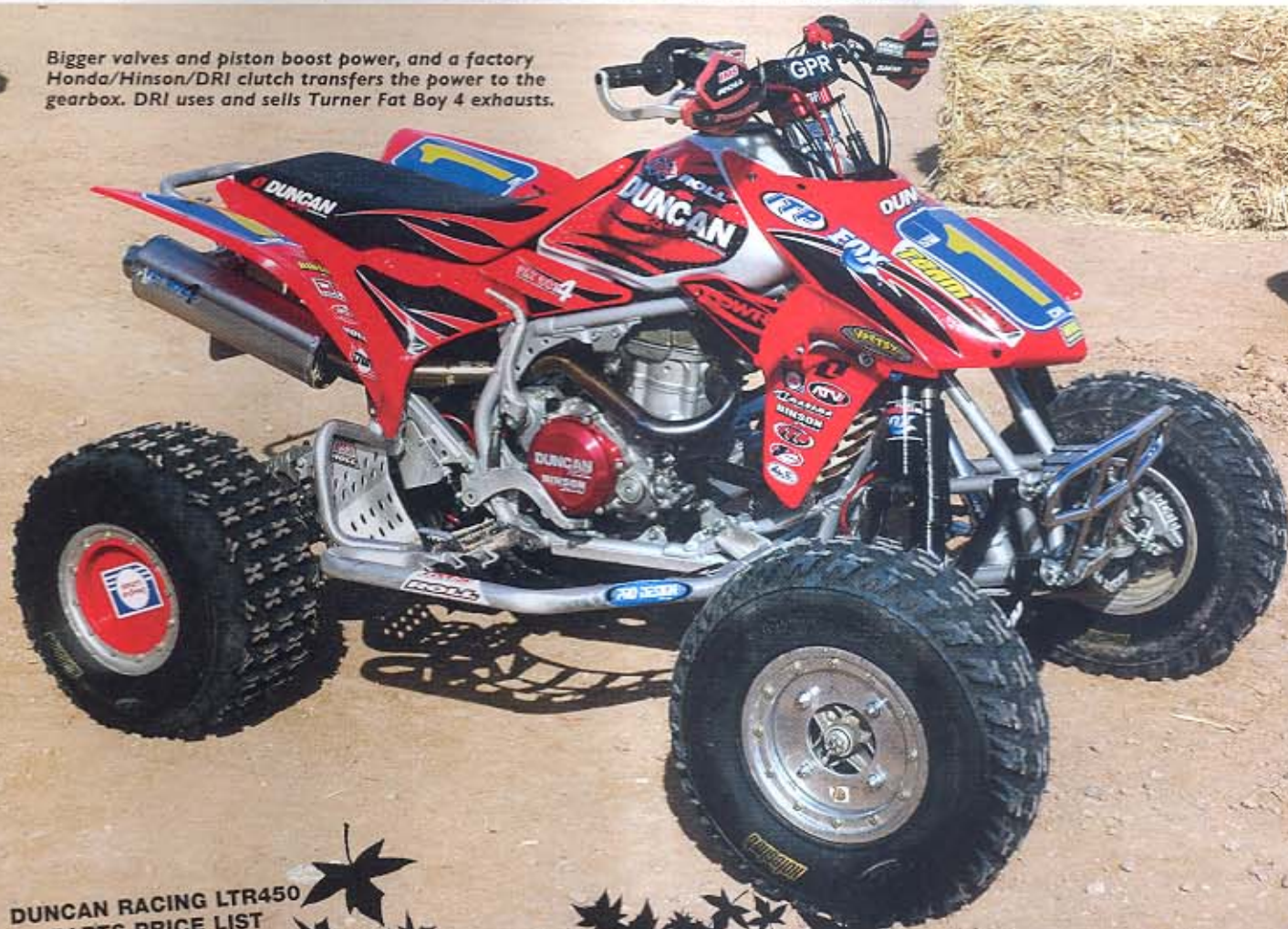
A solid swingarm pivot, countershaft sprocket guard, rock deflectors and full skidplate arm the beast for battle.
