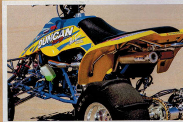
Elka's Stage 4 shocks are thoroughly modern, but most of the other parts on this show-quality Quadzilla could have been on any LT-500R in the 1990s.
