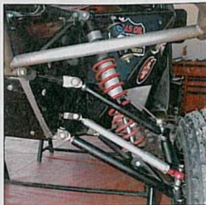
Chromoly A-arms and huge Fox shocks are used on the front of Kyle Hart's Modified Kart. There is slightly more wheel travel on these machines than on the best race quads.
