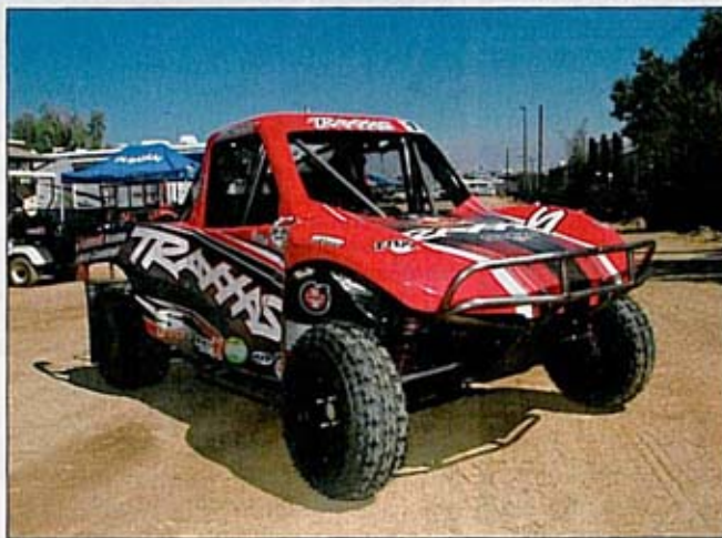
With or without the fiberglass truck body, this Super Kart looks trick. It uses an ATV powerplant, tires, wheels and a similar front end. The body alone sells for about $800.
