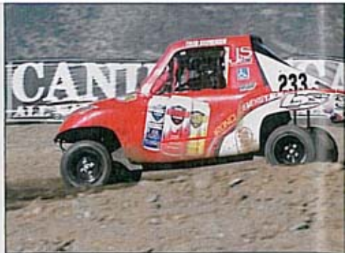
Former ATV racer Jimmy Stephenson's kid, Tyler, competes in one of the entry-level kart classes. These machines feature Honda and Subaru engines with a centrifugal clutch. Used karts like this are priced at around $10,000.
