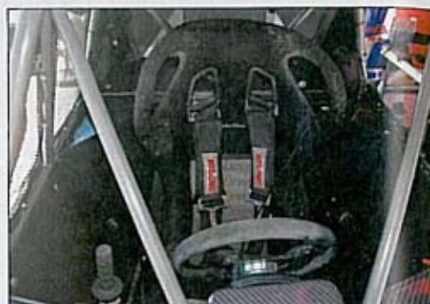
The cockpit of a Super Kart is sized for kids 8 to 15 years old. Being surrounded by a chromoly cage and strapped in with a five-point seatbelt, the kids are pretty safe in the driver's seat.
