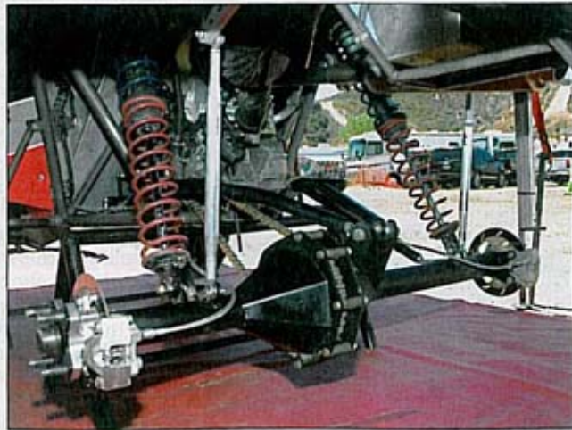
Out back, an amazing center-sprocket-mounted rear end provides the drive on Mitchell DeJong's kart. A winning kart like this will set you back over $35,000.
