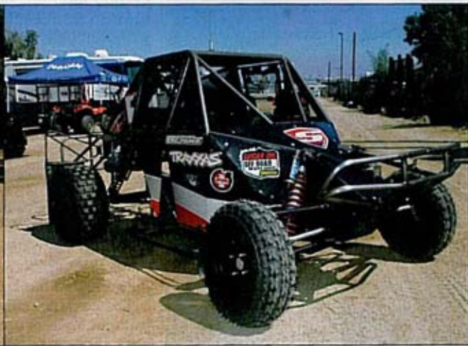
With or without the fiberglass truck body, this Super Kart looks trick. It uses an ATV powerplant, tires, wheels and a similar front end. The body alone sells for about $800.
