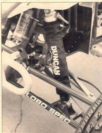
■ The heart of the LOBO chassis is its almost infinite adjustability. Adjustments for castor, camber and toe-in on the front end are quick and easy with the heim joint A-arms. Doug Roll, the creator of the LOBO chassis, has come out with a manual detailing adjustments of the chassis and suspension for varying track conditions.
