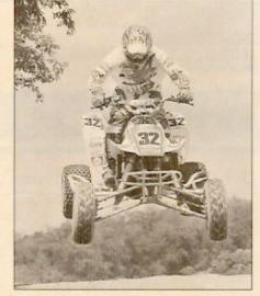
The LOBO chassis' handling was so responsive that it took some getting used to at first. There was absolutely no bump steer whatsoever on the machine and not a hint of pushing in the turns. This allowed the rider to dive for the inside line, even in a bump-infested corner.
