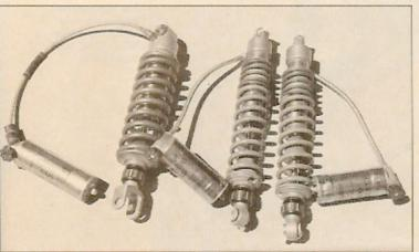
Custom Axis did the shocks on Mark's race quad. They feature adjustable compression, rebound and pre-load on both the front and rear suspension.
