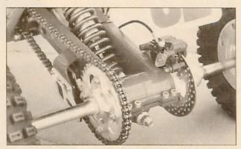
See that nut and bolt just below the middle of the rear axle bearing carrier? That allows you to adjust the leverage ratio on the back end of the LOBO chassis. In order to make tuning the rear suspension easier, future LOBO chassis will use a set-length rod instead of the adjustable version Mark has.
