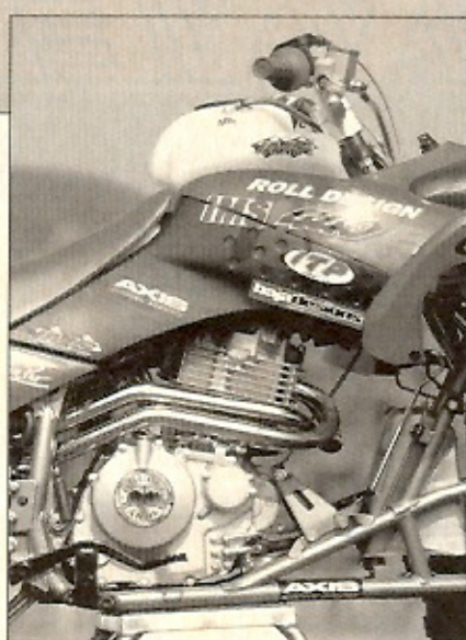
The IMS 440 engine kit consists of bigger bore piston and resleeved cylinder, a hotter cam, ported head and Duncan Racing Double Barrel exhaust system.
