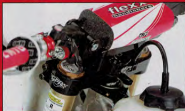
A GPR V-4 stabilizer does wonders for the '09 Honda, whether it's used for MX or off-road.
