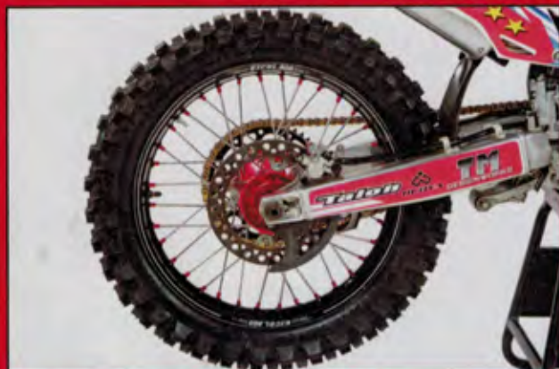
A set of Talon wheels from Dubya helped make the Honda off-road-worthy. Pirelli Scorpion MX tires were used front and rear.
