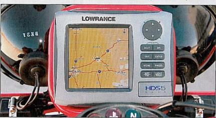
We equipped this 700XX Trail Explorer with a huge Lowrance GPS unit. We could watch speed and track distance all while riding, day or night. This is the same unit many Trophy Trucks use in Baja racing. The mount was installed on the back of our Ricky Stator lights.
