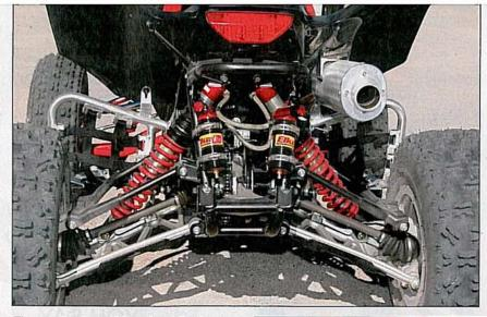
The most unique thing about the twowheel-drive 700XX is its independent rear suspension. Duncan Racing widened it by adding two-inch, aluminum wheel spacers and wide DWT wheels. During our testing, the extra ground clearance allowed us to dominate a local desert race.
