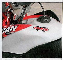
IMS tanks can be ordered with a standard, twist-on gas cap or with a dry brake, quick dump system. On this machine, it was pretty easy to install since the stock fuel pump is located outside of the tank.
