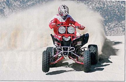
The heavy 700XX even works well in the sand with the Duncan Racing upgrades. We slowed down the slow speed compression on the rear Elka shock to make it perform as well as a straight axle machine. You can see a complete test of a sand dune-equipped 700XX at www.dirtwheelsmag.com.
