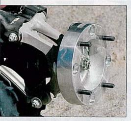
Two-inch-wide aluminum wheel spacers were installed on the rear of this machine to widen its stance. The Elka shocks added preload to offset the increased leverage.
