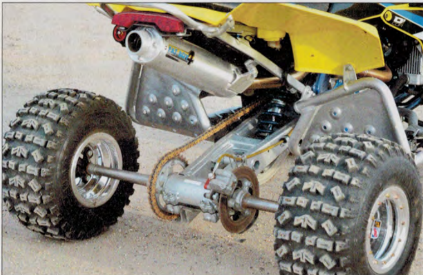
Out back, we installed a Lone Star Racing axle, bearing carrier and RK chain. It rolls smoother than stock, and we're confident it's way stronger too. The Duncan Fat Boy exhaust is center-mounted like the stocker and sounds great to the rider. It might be a little loud to those guys you pass.
