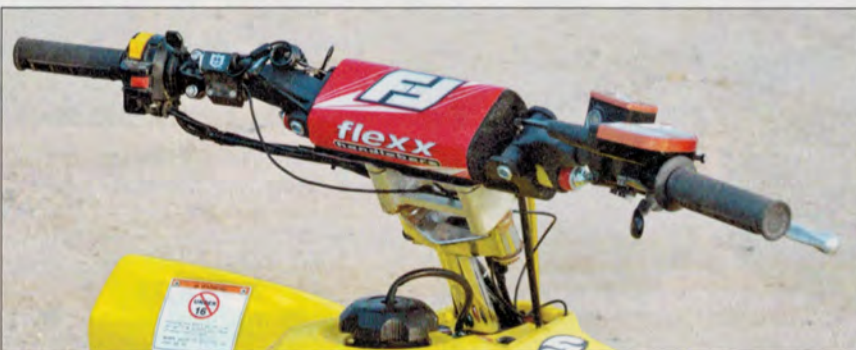
Any little tricks you can do to fight rider fatigue is well worth it if you want to go fast for a long time. These Flexx bars from Fasst Co., along with a GPR stabilizer, attach to the Roll Anti-Vibe stem almost give you the same advantage as installing aftermarket shocks.
