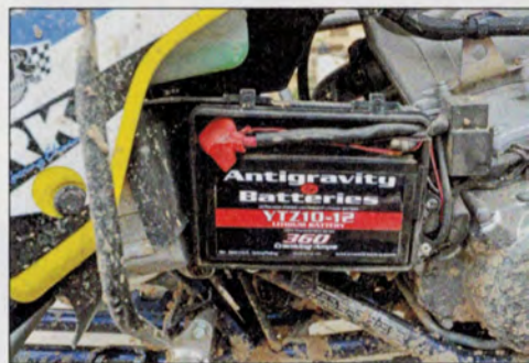
Today's fuel injected quads require a strong battery in good-working condition to power all the electronics. This Antigravity lithium-ion battery does that all while weighing half that of a lead-acid product.
