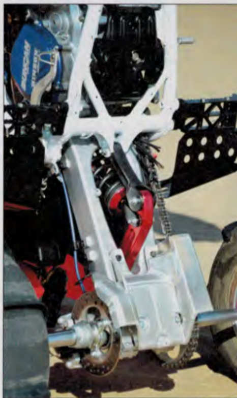
The stock swingarm was left on this Honda, but it was outfitted with a Elka shock and linkage. The small aluminum skid plate was mounted up for those rockier rides away from the dunes.
