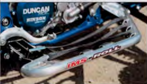
The IMS-Roll nerf bars and pegs were comfortable and strong, but we missed the heel guards.
