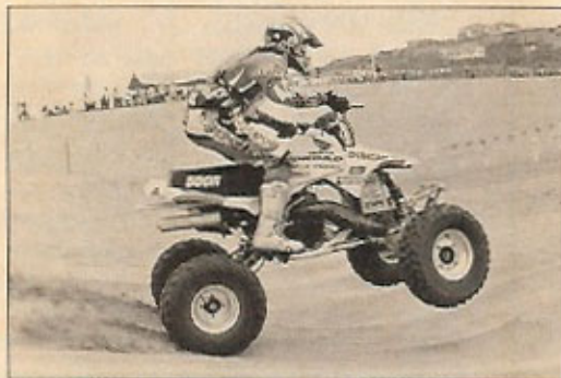
The DRD&D (Doug Roll Design & Development) 500R is the result of combining a Honda CR500 motocross engine inside a Doug Roll chassis and bolting on an array of wheels, tires, gas tank and parts to come out with a high-performance hybrid.
