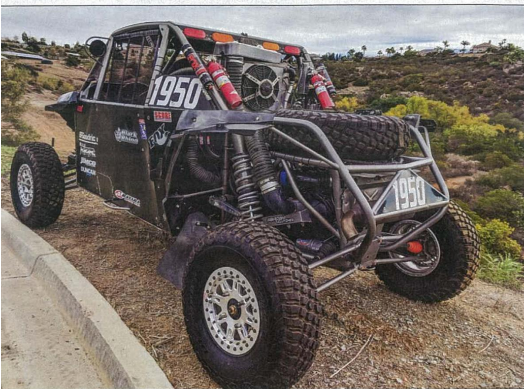
The rear-mounted CBR radiator greatly increases cooling capacity, protects the radiator from roost and impact damage, and the custom ducting boosts transmission cooling.
