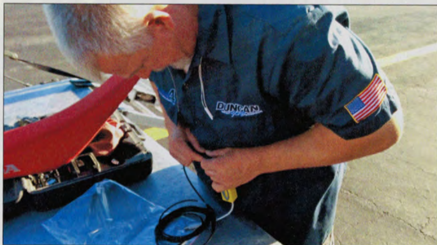
If you have the know how to map out your own ignition curve, the Vortex ECU has one setting that is open to programming by the end user. The programmer hooks up to a laptop and sells for $500.
