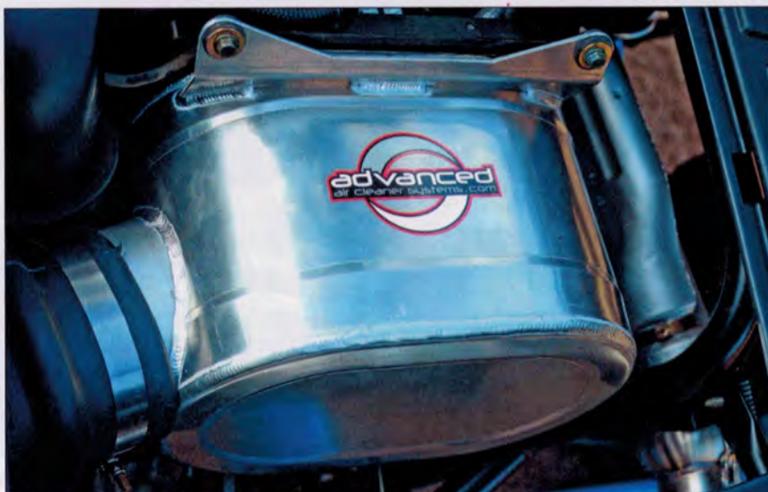
The Advanced airbox breathes better than stock. Unfortunately, that makes the RZR run even leaner, and it's difficult to bring more fuel into the equation with the stock ECU.
