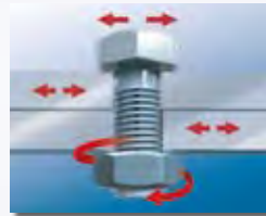
Vibration and loosening
