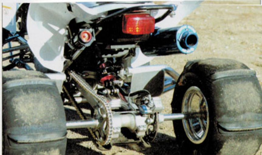
■ An adjustable, rebuildable Elka rear shock replaces the basic, non-rebuildable stock shock.
