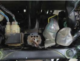
**Step 6:** Carefully plug the 33 Way connector onto the VORTEX ECU and push firmly until the locking tab clicks. Use the smaller zip ties provided to secure any lose wiring.
