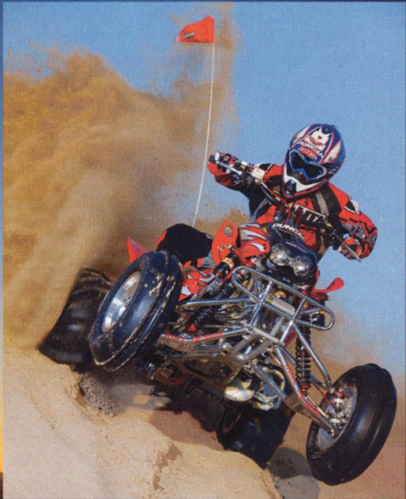
Above Getting all the ponies to the sand was managed with ease by ITP Sand Stars mated to Douglas Quad-Rok wheels. We ran the tire pressure at 8 psi in the front and 6 in the rear.
