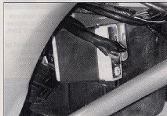
The Vortex ignition mounts in the stock location and plugs into the stock wiring harness. The small white dial on the bottom is for fine-tuning the main adjuster mounted on the handlebars.
