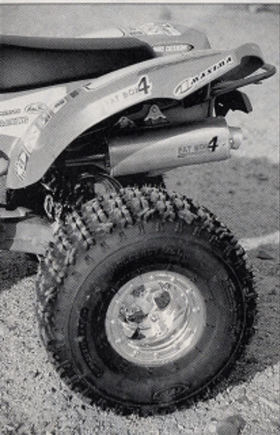
Douglas heavy duty shamrock aluminum rims with ITP Holeshot XCT knobbles held up extremely well to the rough desert conditions. Only one flat was recorded during the race.
