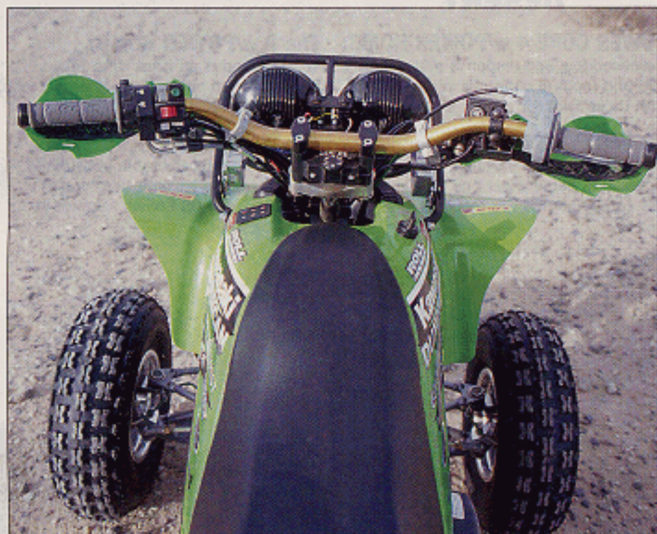
A set of Tag 2 alloy handlebars was added to the big Kawie to help smooth out the ride for the six-member team.
