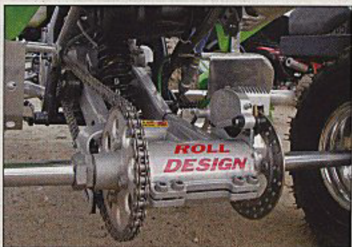
The rear disc holder is modified to accept a Honda 250R rotor for increased ground clearance and the custom calliper from ATV Innovations keeps the brakes cooler.
