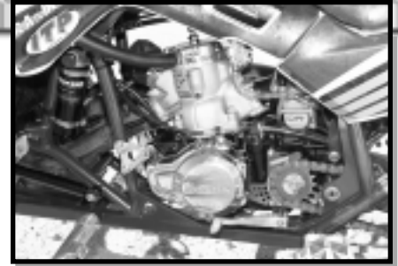
The Duncan Racing PC 2000 Power Cylinder (as used by Spader) provides a relatively simple, pre-ported, bolt-on upgrade for Honda ATC250Rs and TRX250Rs from 1985 to 1989.
