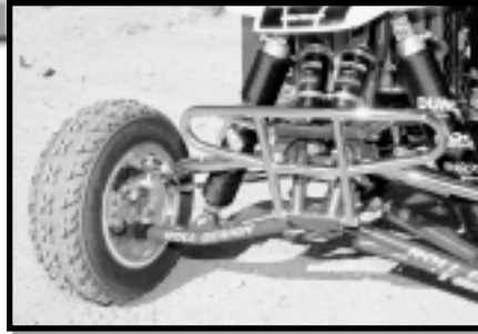
The team plans to run these Holeshot MX front tires exclusively for the 2001 season. Note the unique shape of the Lobo lower A-arms, as well as the 400EX spindles and brakes.
