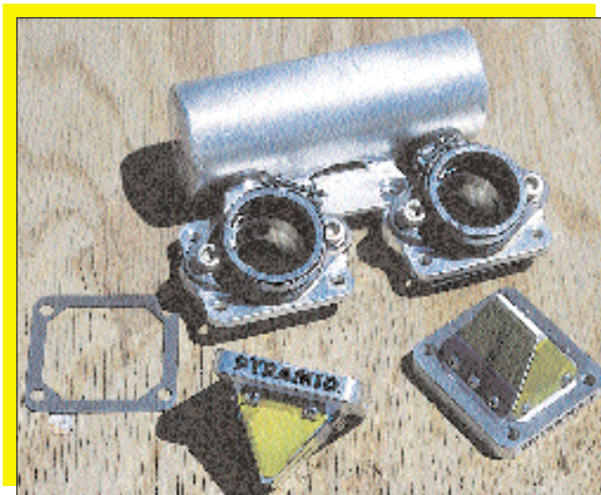
The Master Flow intake manifold and Pyramid reed valves really boost throttle response.
