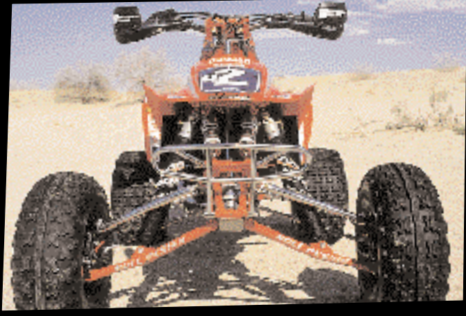
Up front the 51-inch wide quad has Roll Design +3 A-arms and steering stem, Custom Axis suspension, and Tag Metals CR500 handlebars.
