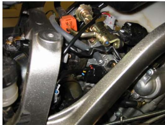
**Step 5:** Lift the petrol tank to one side and unplug the grey 2 Way Fuel Injector connector. Plug the Blue 2way connector from the EFI Interceptor into this connector.
