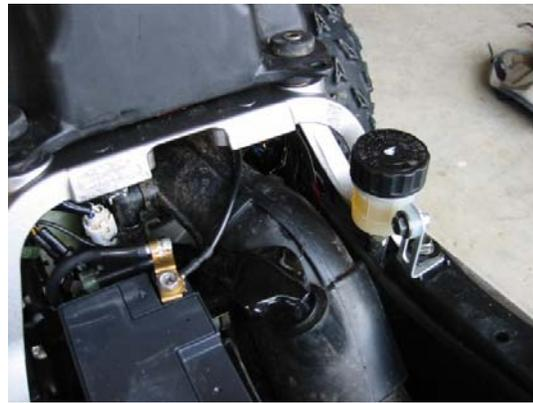
**Step 2:** Mount the EFI Interceptor in behind the tool tray under the seat. Use the Velcro provided to secure it in place. Note: Always clean the plastic surface with alcohol before applying the Velcro.
