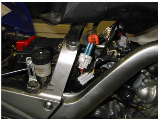
**Step 8:** Plug in the Grey 3 Way connector from the EFI Interceptor harness into the Black 3 way connector previously unplugged from the Throttle Position Sensor.
