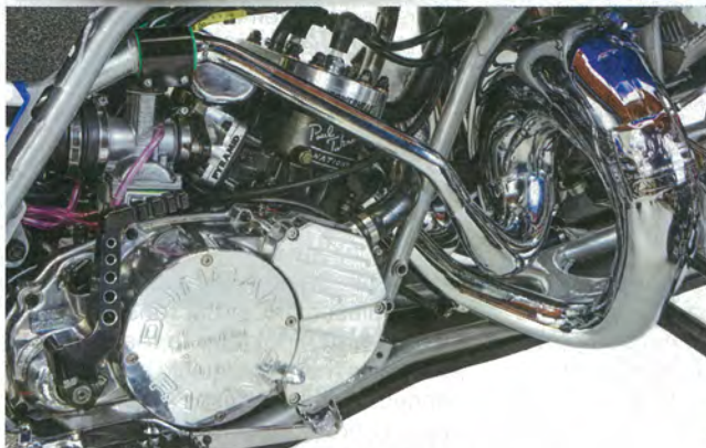
The Paul Turner pipes were triple-chrome-plated to resist abuse. Plenty of other parts were polished or chromed for that custom look.
