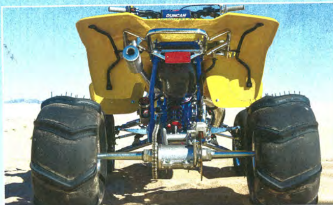
Left: Duncan Racing has 20/20 hindsight. It added engine and suspension performance, including a new custom swingarm, but kept Suzuki's good stuff that was good then and now.
