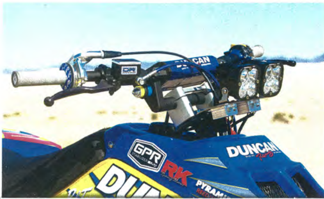
Left: Owner Danny Franco rides this legend, so he opted for a Flexx handlebar with modern controls and modern lighting from Baja Designs on a custom Duncan mount.
