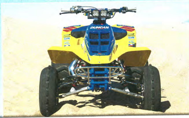
Right: Aside from the Elka Stage 4 shocks and premium finishes, much of the front end is as Suzuki built it. It still works just fine. The engine is not quite so stock!
