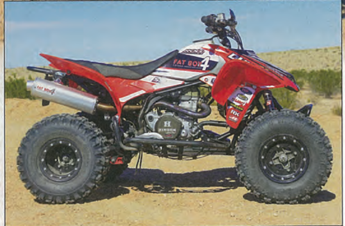
Peek under the rear of the machine and you will see that it doesn't use a stock linkage but one specific to the Elka shock. The Roll Design nerf adds safety and peace of mind.
