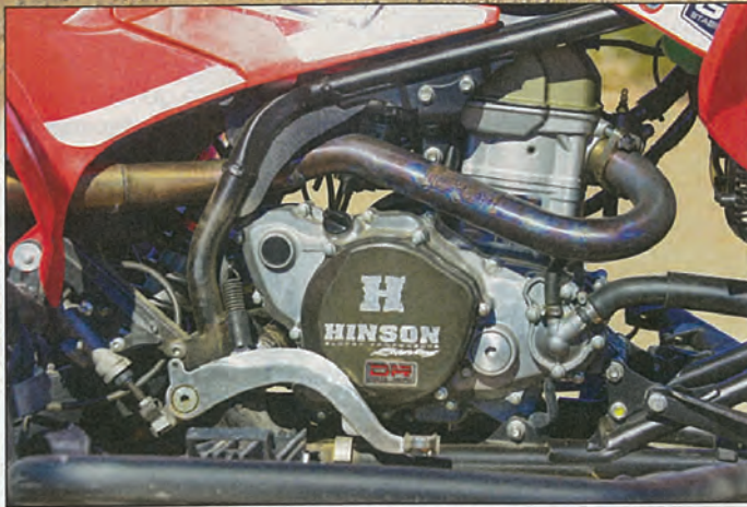
Engine performance comes from intake, exhaust and Vortex CDI mods. Internally, there is more compression, big valves, porting and a cam. It runs hard.
