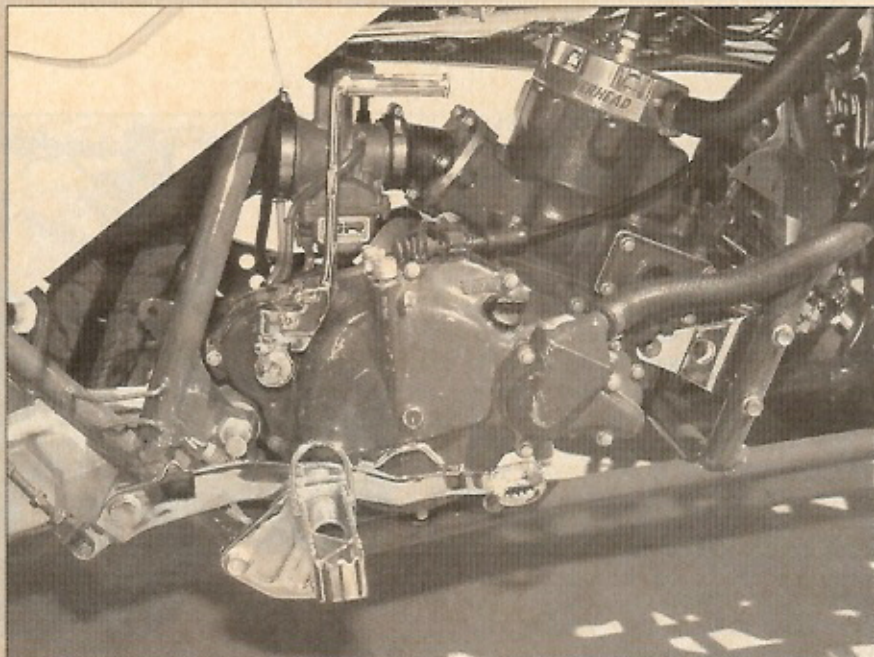
Duncan Racing's Eliminator kit, with Powerhead and 39mm Keihin PWK carb, cranks out good low-end and midrange for the trails and more technical riding.
