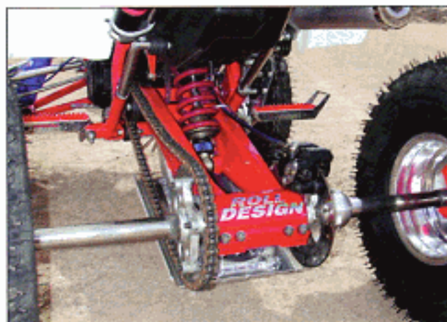
The Golden West machine's full-race rear suspension includes a fully adjustable Custom Axis shock and Roll Design swingarm.
