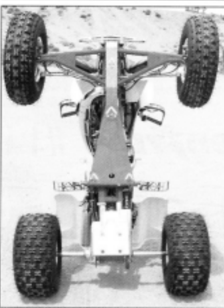
Golden West skid plates protected the machine's underside from the miles of rocks on the Nevada 1000 course.
