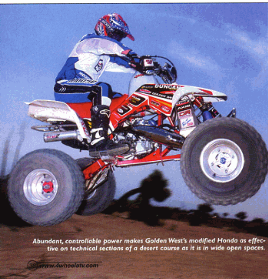
The Golden West machine's full-race rear suspension includes a fully adjustable Custom Axis shock and Roll Design swingarm.
