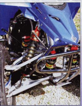
Elka remote reservoir shocks make a dramatic improvement in the Blaster's handling. Unlike the stock shocks, they're rebuildable and tuneable.
