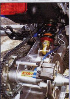
The Elka rear shock has a larger shaft and body than the stock unit.
