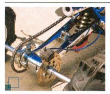
Suspension is often overlooked on duner Banshees, but not here. The Duncan project has top-of-the-line Roll Design A-arms up front and a +4 Laeger swingarm in the rear, with Elka elite shocks all the way around.
