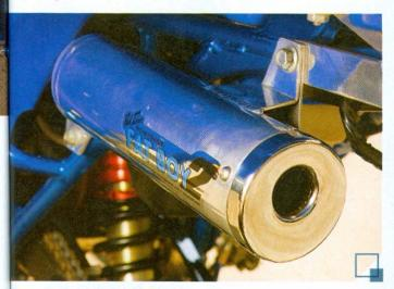
Simple and effective. The DRI Banshee's twin Fat Boy 2 silencers quiet the combustion and give the two-stroke a deep, healthy roar. The polished end-caps are available as an upgrade, and DRI also stocks turn-downs and spark arrestors for regulated riding areas.
