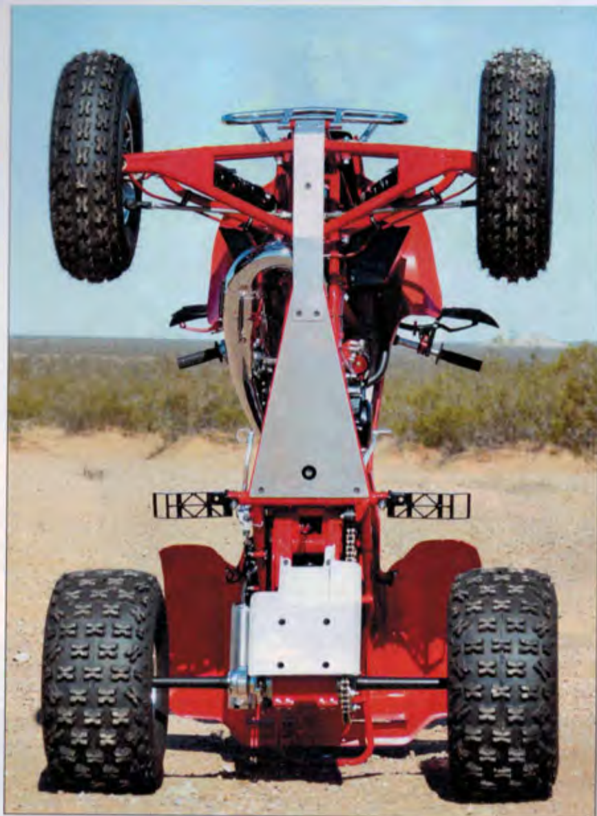
Doug Roll custom-made the skid plates for the Lobo frame. With a chassis this rare, you want to protect it well.
