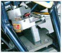
An Elka steering damper helps to tame the high-speed swap out of the handlebars. It is fully adjustable and rebuildable.
