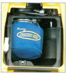
A Pro Design air filter and Outerwear cover helps to provide a steady supply of clean air to the DRI motor.
