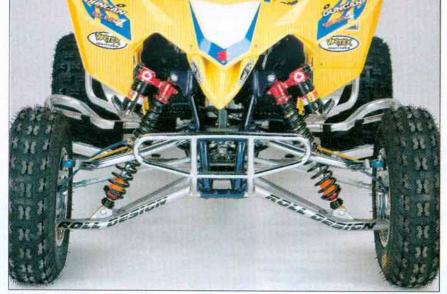
With the IMS/Roll Design front A-arms and Elka long-travel suspension at both ends, the DRI LT473 has the handling chops to handle the increase in useable horsepower and torque.
