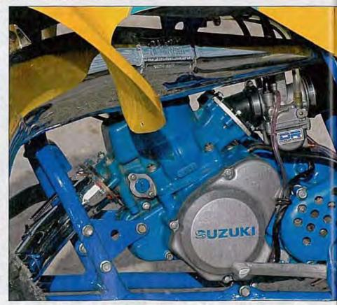
What we did lose with the two-stroke was a lightweight engine. It is also easier to work on than a modern-day race motor. Even though it has 200-less cc, horsepower differences are in the low 30s for the two-stroke and low 40s for the thumper.
