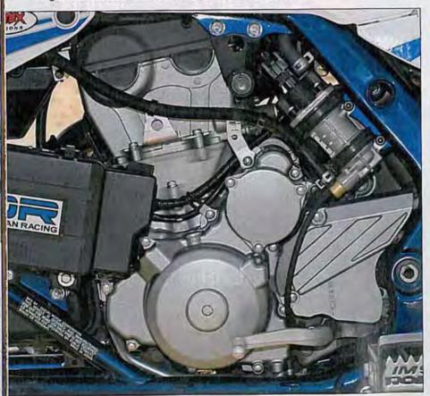
Four-stroke engines take up a lot more room in an ATV chassis. An external oil tank, battery and fuel pump are added components. A smaller battery can be installed along with a kick starter
