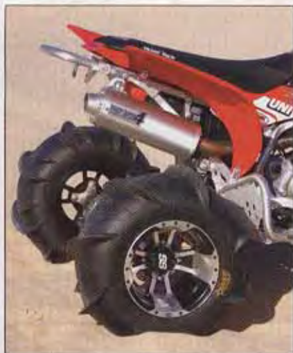
ITP's slick looking SS Series wheels, along with their Sand Star tires gave our machine solid hook up in the dunes. The Duncan Fat Boy 4 exhaust picked up the powerband, especially off the very bottom and gave us more top end.
