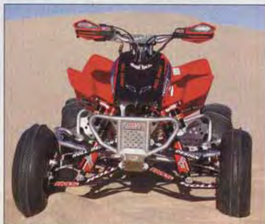
Making the front and back ends much wider and better working was accomplished by installing a set of Roll Design gull-wing A-arms and Elka Elite shocks.
