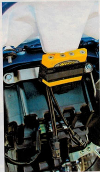
The Vortex X10 ECU mounts where the stock unit usually resides. It's simple to adjust each knob by inserting a flat-blade screwdriver through the top of the plastics where the seat latches on.
