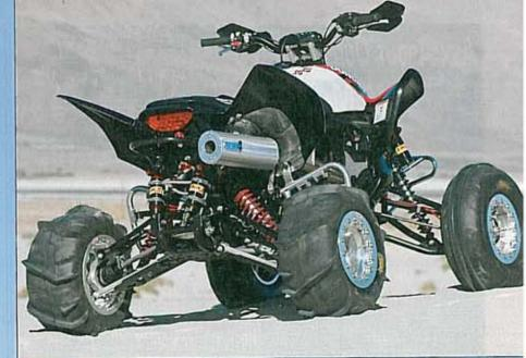
Out back, MTA wheel spacers provided a 2-inch width extension on each side. This allowed Duncan to install 10-inch DWT wheels instead of using the stock 11-inch wheels, which no one sells paddle tires for.
