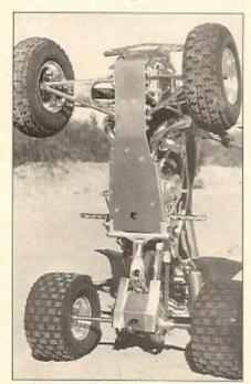
OMF and Duncan Racing offer excellent engine skid plate protection that has proven itself time and again in the Baja 500 and 1000.
