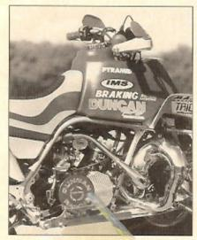
IMS makes a handy replacement plastic gas tank for the Banshee that holds 5.6 gallons for long-distance cruising. The Paul Turner midrange Banshee pipes gave the machine a smoother midrange-to-top-end power spread.
