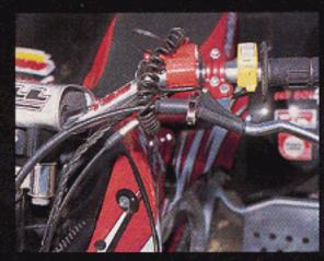
We loved the ergos on the Honda and we like the GPR stabilizer for any type of riding. The Vortex thumbswitch just inside the handgrip selects between two ignition curves.
