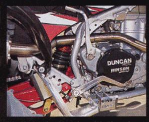
We rode the Honda with the single-shock linkage in the rear and were impressed. Since this photo shoot, Elka has released a duallink setup for even more travel and more resistance to shock fade under race conditions.
