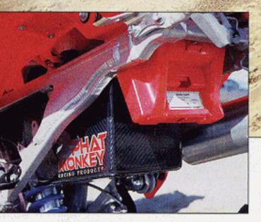
A new company call Phat Monkey is working closely with Avenger on developing carbon fiber parts for ATV's. Their first product for the TRX450R is this custom airbox.
