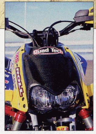
If carbon fiber is in your budget, than Quad Tech has a Honda nosepiece that still allows you to run your stock headlights. Carbon fiber is becoming a must have over chrome these days.
