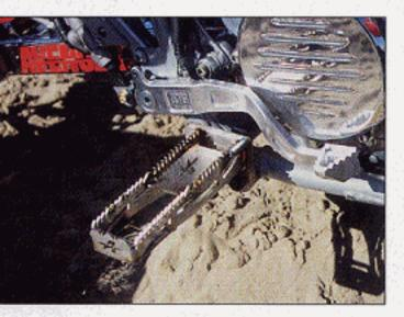
One of the coolest parts on the Avenger quad was the pair of titanium footpegs. They would have been even better attached to some sort of heel guards.
