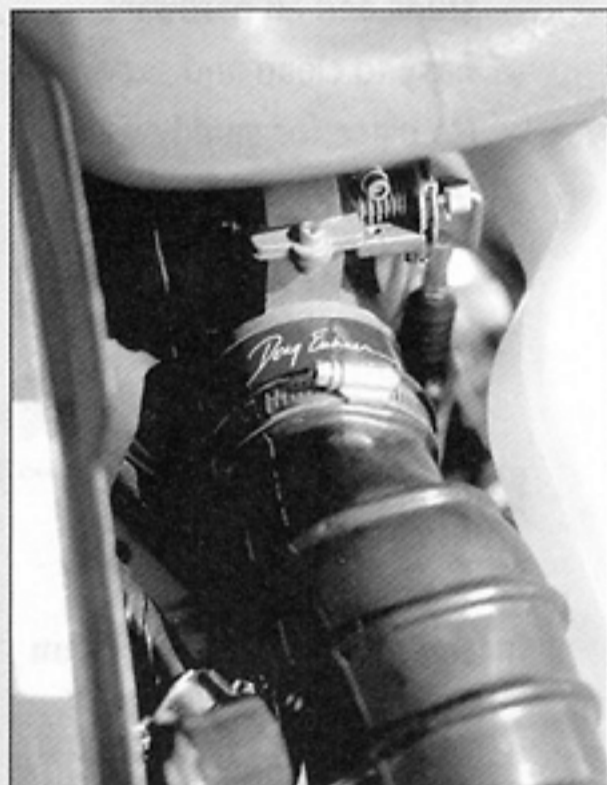
How many guys have their own signature carburetor? The Edelbrock 38mm carb on the Duncan 440EX is....you guessed it, a Doug Eichner signature model.
