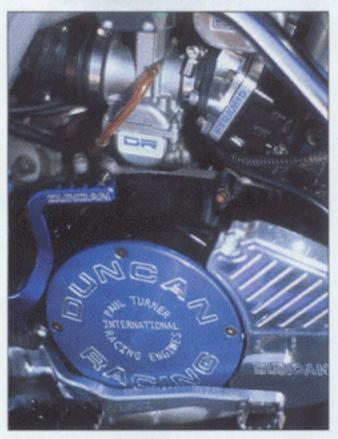
A removable DR clutch cover allows for easy servicing of the Banshee clutch plates. A Hinson Racing clutch basket replaces the stocker and helps keep the clutch alive with the increased horsepower.
