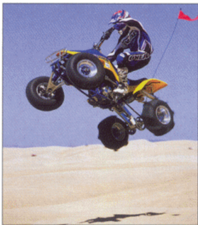
Brian Radovich launches off a Pismo dune aboard the Duncan Racing LT500. We upgraded the stock Suzuki suspension with a set of Ohlins shocks up front and a revalved Suzuki shock on the back end. The suspension mods made it a much better all-around race and play machine.
