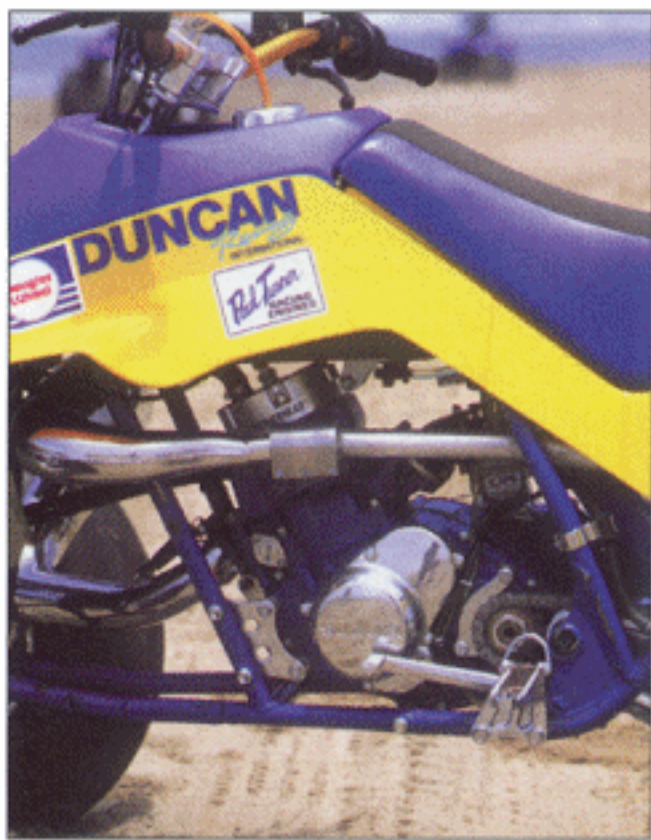
A Duncan Racing PTR National engine kit with a Powerhead and DR Super Flow carb mod gave our LT500 a major boost in power. The mighty liquid-cooled two-stroke is still a potent weapon in the dunes.
