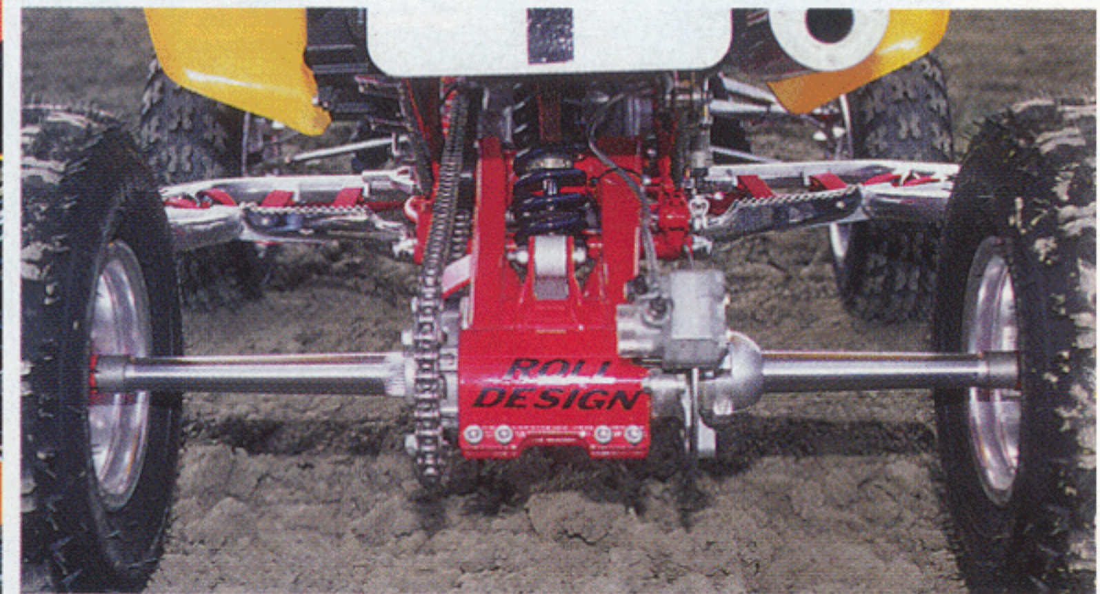
Just as it does for the front end, Roll Design offers a rear end suspension kit. A linkage-free swingarm is matched to a custom Axis shock. That's a 48-inch Dominator Axle with a Millennium carrier.
