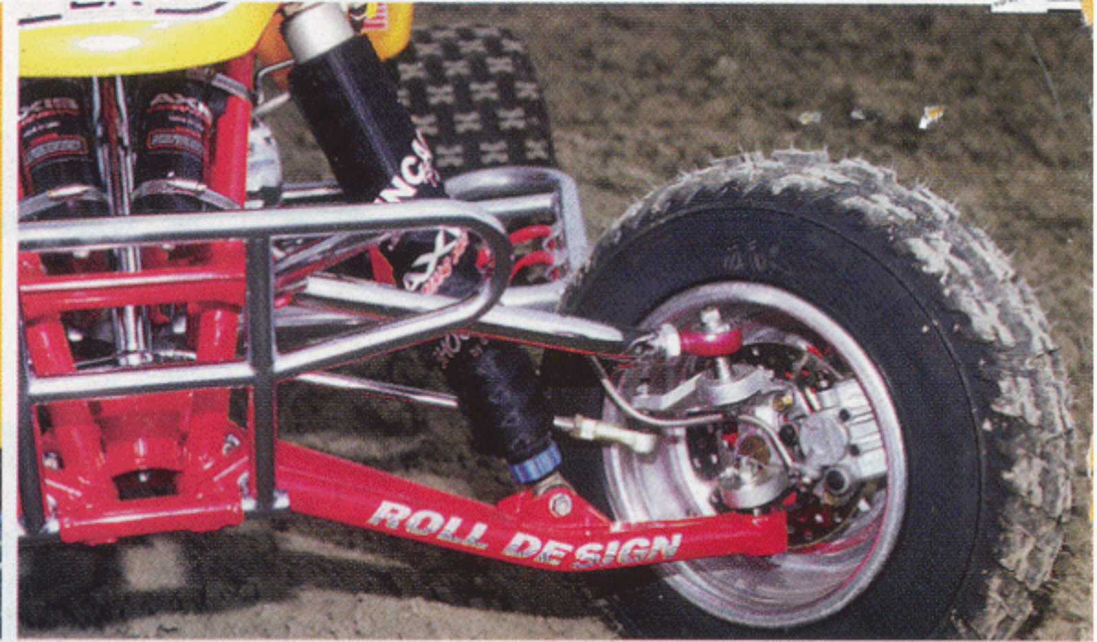
The Roll Design Lobo II front end kit adds needed stability to the 400EX and offers vastly superior suspension action. The kit bolts onto a stock frame and includes A-arms, specially made Axis shocks and tie rods.
